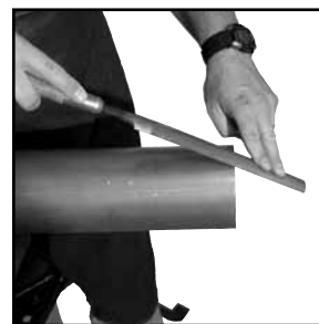
Figure 4: Deburr outside diameter using a half-round file
