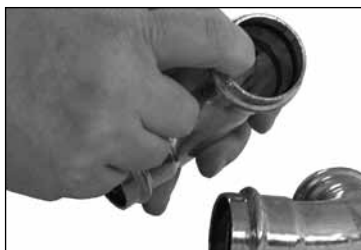
Figure 2 — Check for EPDM Seal
