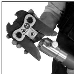
Figure 7: Placement of adapter jaw into the tool
