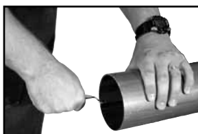
Figure 3: Deburr inside diameter deburring tool
