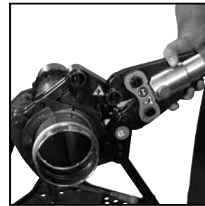
Figure 8: Placement of adapter jaw into pressing chain
